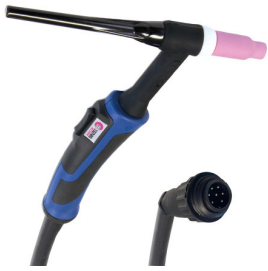
595038202 TIG TOORTS SR 20 DB -T50 - 4M - AMPHENOL KUNSTOF CONNECTOR - 7PIN - LIQUID
