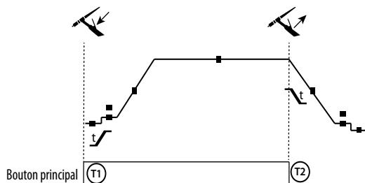
T1 - The main button is pressed, the welding cycle starts (Pre-Gas, I\_Start, upslope and welding).
