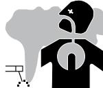
The fumes, gases and dusts emitted by welding are harmful to health. Sufficient ventilation must be provided and an additional air supply may be required. An air-fed mask could be a solution in situations where there is inadequate ventilation. Check the extraction system's performance against the relevant safety standards.
