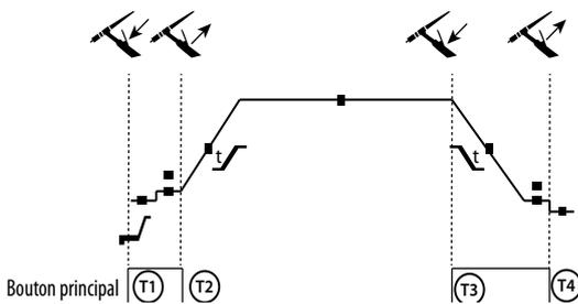
T1 - The main button is pressed, the cycle starts from Pre-Gas and stops at the I\_Start phase.
