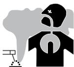
The fumes, gases and dusts emitted by welding are harmful to health. Sufficient ventilation must be provided and an additional air supply may be required. An air-fed mask could be a solution in situations where there is inadequate ventilation.
