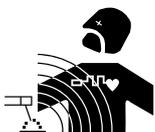
An electric current passing through any conductor produces localised electric and magnetic fields (EMF). The welding current produces an electromagnetic field around the welding circuit and the welding equipment.
