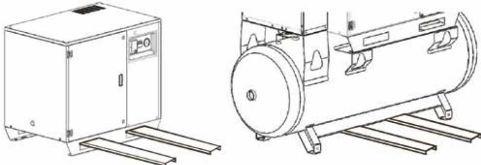
The compressor without air tank must be lifted with a transpallet or a truck with appropriate capacity. In the same way the compressor with air tank (see fig. 9) must be lifted. The weight is shown in the section 3.2 Technical Features.
